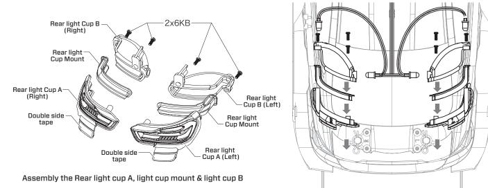
Use screw 2x6KB fixing on the car body and install the LED lightAssembly
