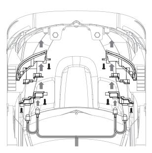
Use screw 2x6KB fixing on the car body and install the LED lightAssembly
