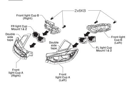
Assembly the Front light cup A, light cup mount & light cup B
